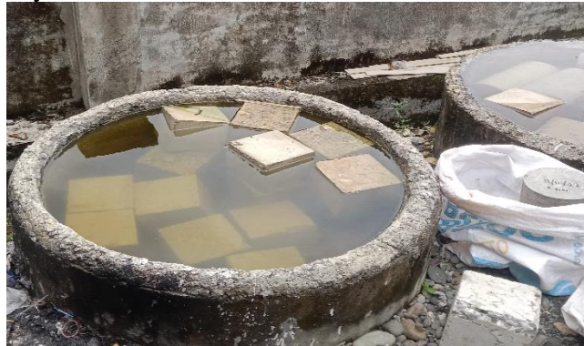
Figure 2.4 Treatment of cube specimens (15 x 15 x 15) cm
