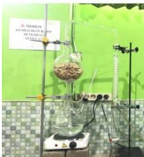
Fig. 1. Image 1. Distillation of Red Ginger Essential Oil ( figure caption )
