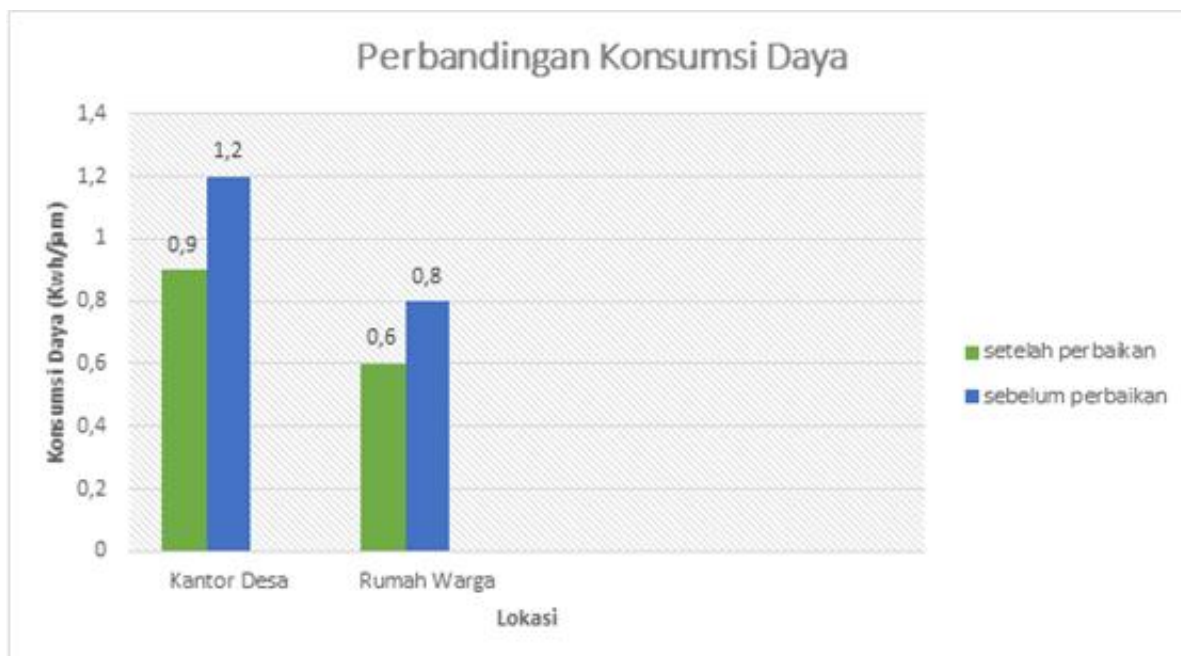
Figure 3. Comparison Chart of Power Consumption Before and After Repair
