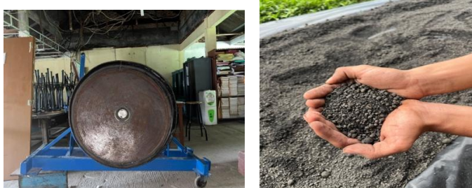
Figure 2. Granulator Machine and Puler Granules as Organic Fertilizer
