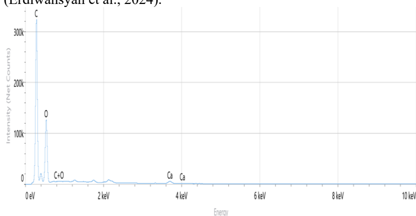
Figure 3. EDX Graph of Palm Strach Waste Ash
